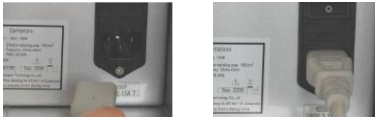
Forth step: Insert electric power cord into power cord connector, and switch on.
